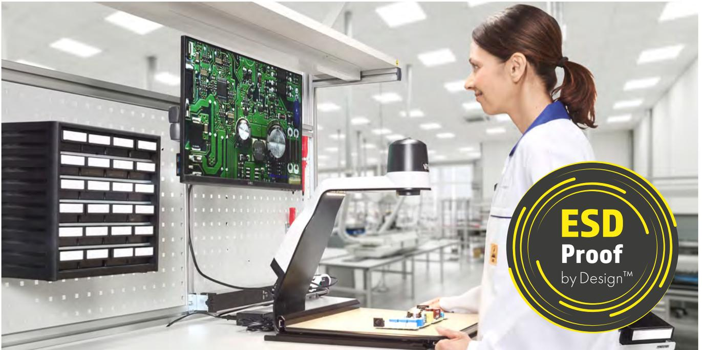
Manufacturing or handling electronic components and products requires protection from ESD, electrostatic discharges. Even the smallest ESD can cause major damage to sensitive components, weaken the end-product's durability, or change its functionality. Costly ESD damages can be avoided by building an ESD protected area (EPA) where ESD workstations play a crucial role.
