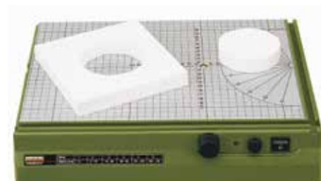
Crosscuts are achieved by means of a simple yet efficient solution: secure drawing-pin to table by means of tape, it serves as a fixed centre.
