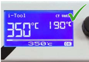
340 – 360 °C for lead-free solder
