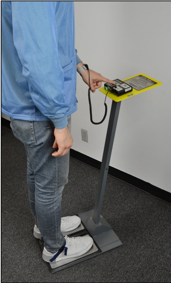
Figure 13. Using the 19271 Combo Tester X3 with Stand
