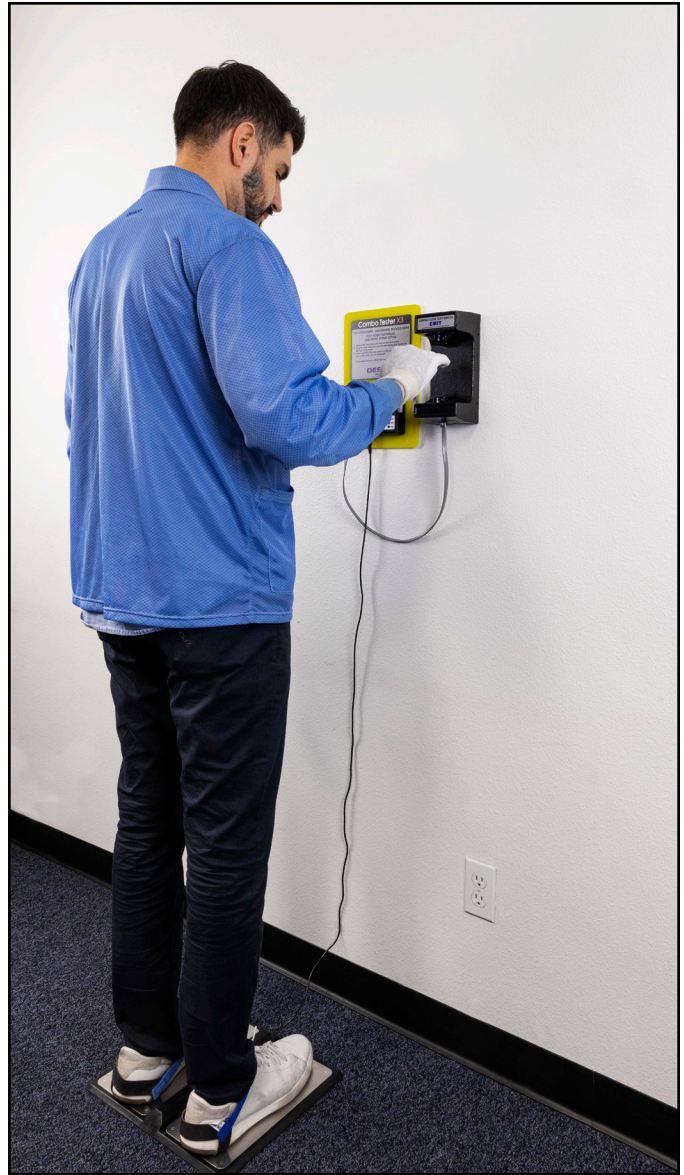
Figure 5. Using the Contactless Test Switch to perform a footwear test with the Combo Tester X3
