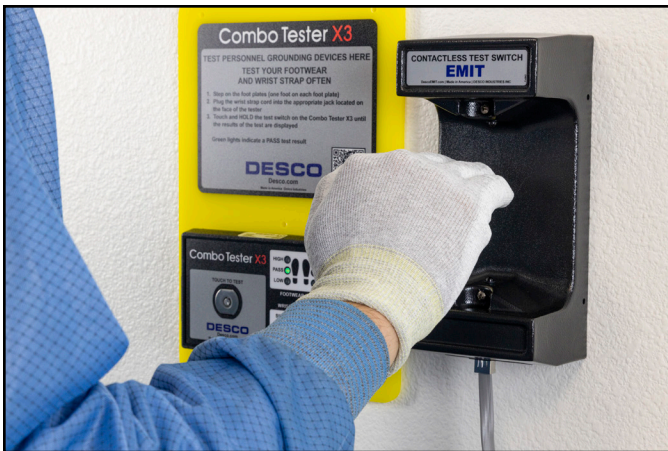
Figure 4. Using the hand to trigger the infrared sensor in the Contactless Test Switch to perform a test with the Combo Tester X3
