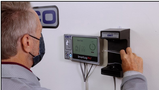
Figure 6. Using a proximity badge to trigger the infrared sensor in the Contactless Test Switch to perform a test with the SmartLog Pro® 2
