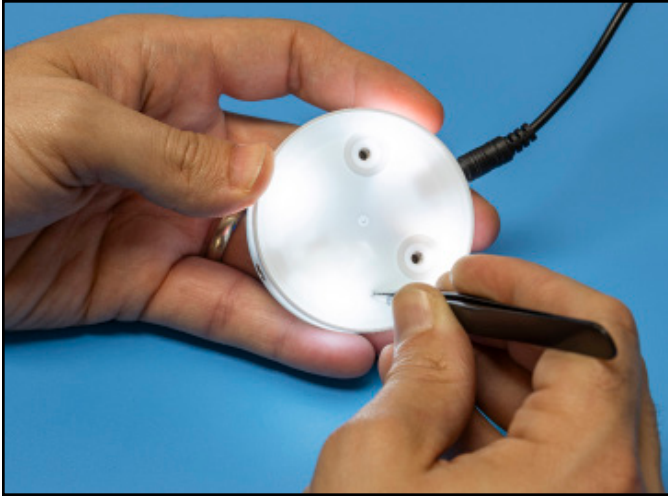
Figure 7. Using the set switch to disable the worksurface monitor circuit
