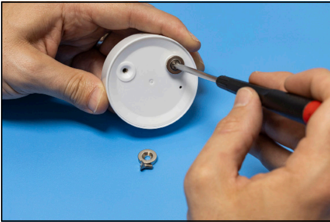
Figure 8. Installing the Desco 19344 Ring Magnets
