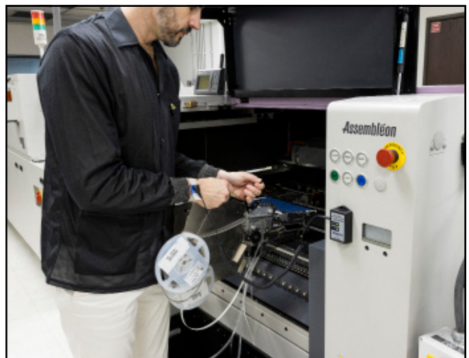
Figure 9. Using the Multi-Mount Continuous Monitor at a machine station
