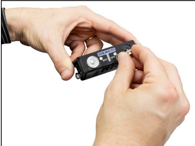
Figure 6. Installing the 10 mm ParkSnap™ to the 19337 Multi-Mount Continuous Monitor
