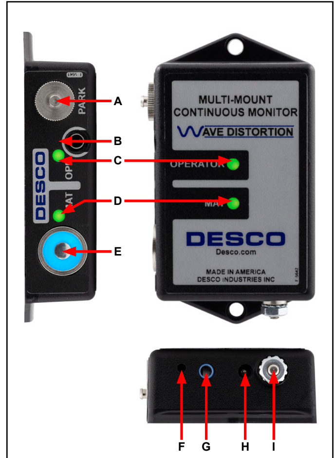
Figure 4. Multi-Mount Continuous Monitor features and components
