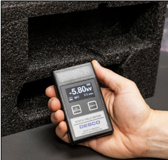
Figure 7. Using the Static Field Meter to measure foam
