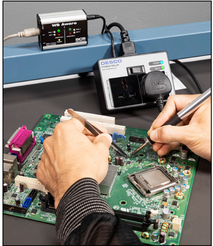
Figure 6. Using the Universal Power Relay with the WS Aware Monitor
