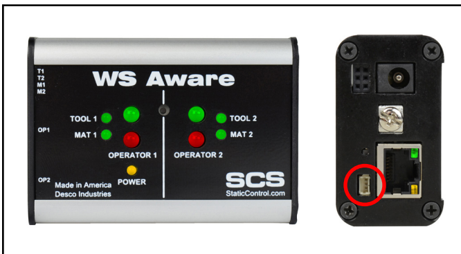
Figure 3. Power relay connector on the WS Aware Monitor
