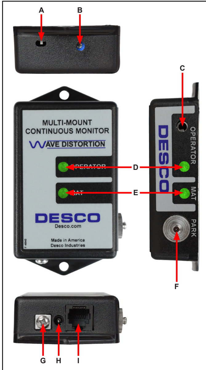
Figure 4. Multi-Mount Monitor features and components
