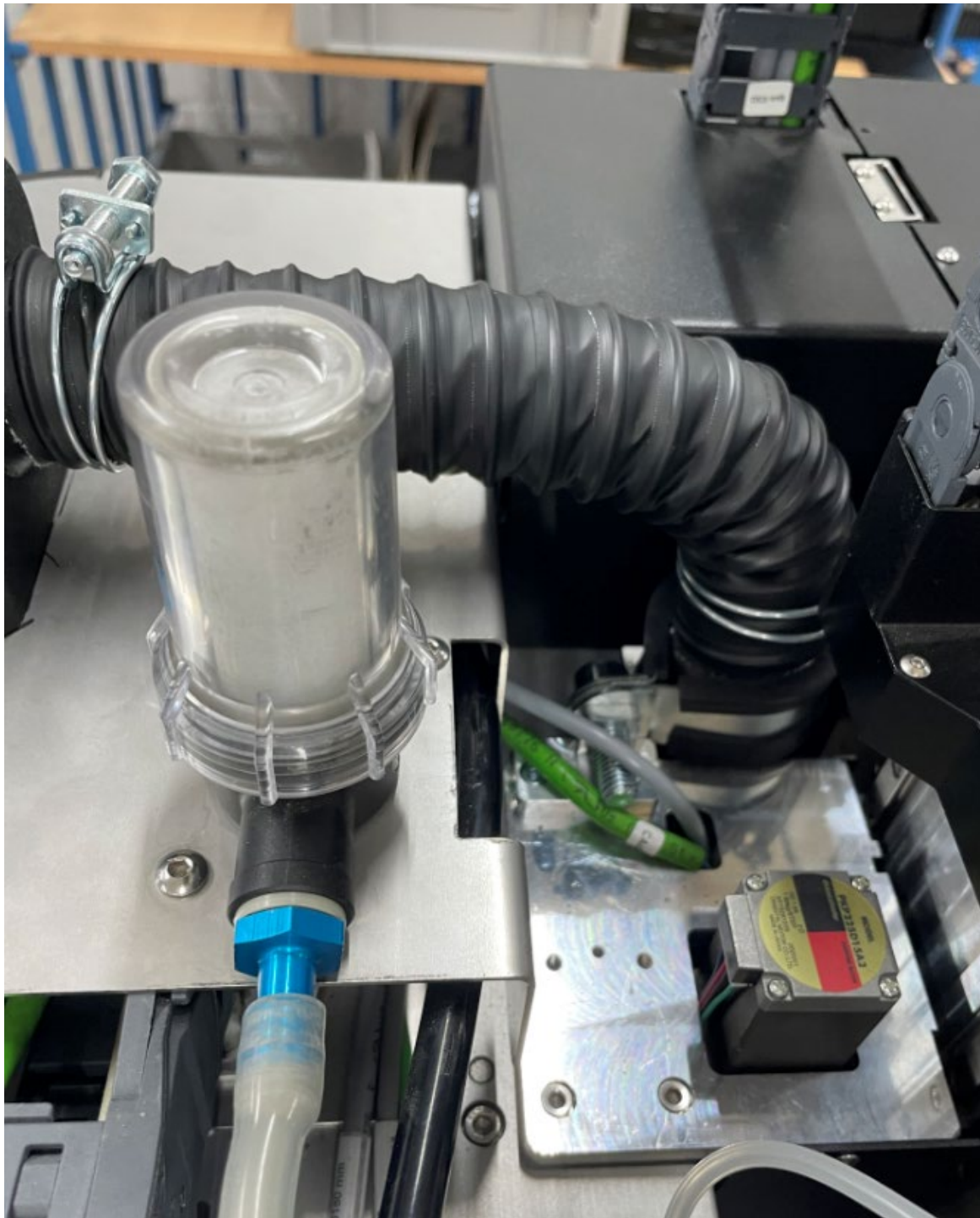
Fig. 2: Mounted solder fume extraction on the Reworksystem HR 600 XL
