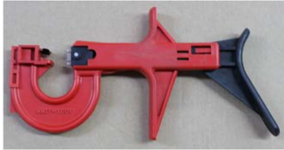
Fig. 14: Crimping tool for pressing in the cables for MAS-CON® female multipoint connectors with a 2.54 mm grid dimension.
