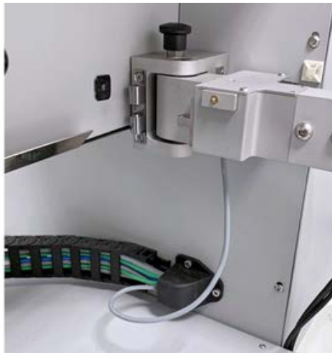
Fig. 15: Cable routing outside the housing, picture after assembly completion.
