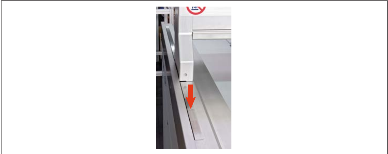
Fig. 54: Oiling sliding surfaces
