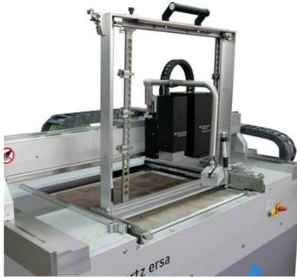
Fig. 16: PCB frame swung into the vertical position
