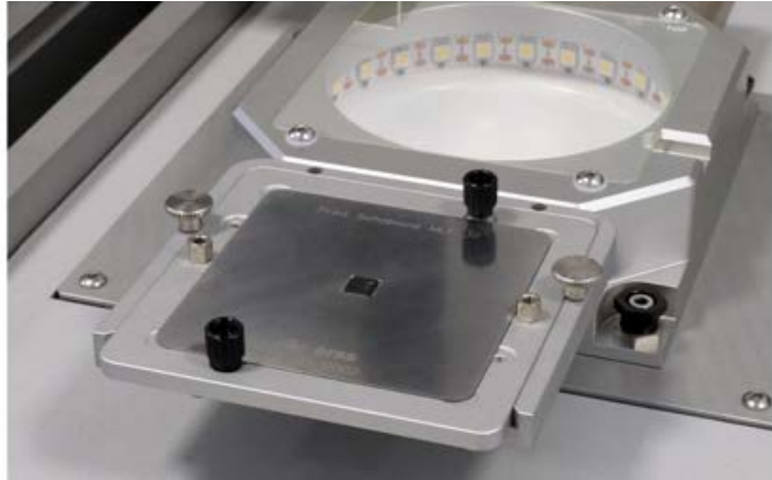
Fig. 48: Example picture: The solder paste-coated component is inserted into the print stencil and slid into the framed stencil
