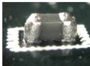
0402: bulbous solder joint
