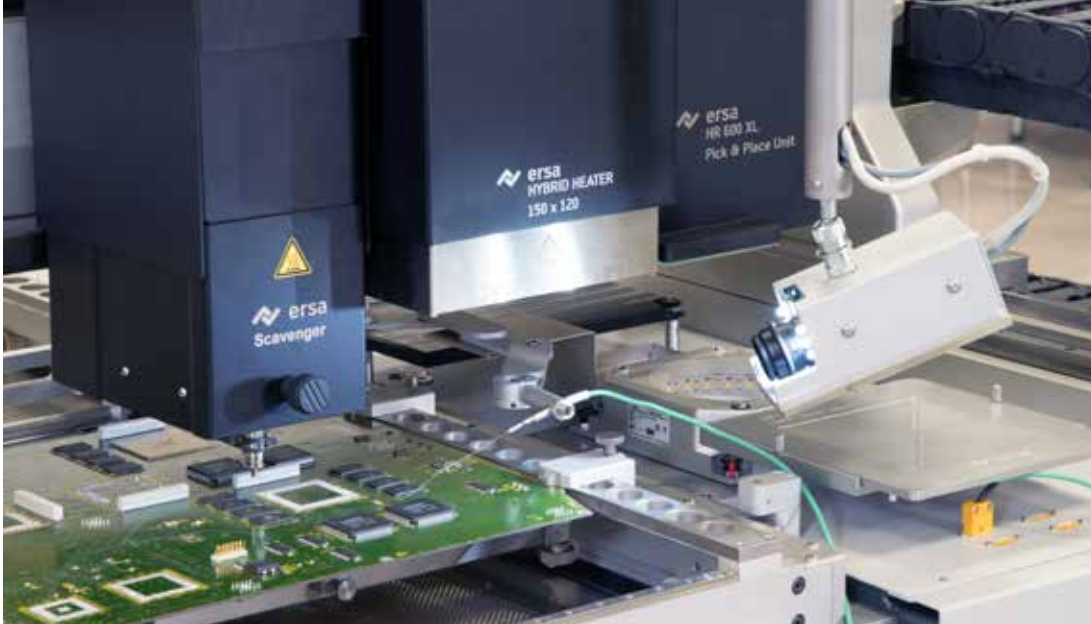
Automatic processing of large assemblies, including residual solder removal and RPC camera
