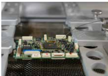
Flexible board holders adapt to size and structure of an assembly.
