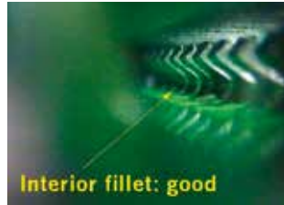
PLCC – interior fillet inspection
