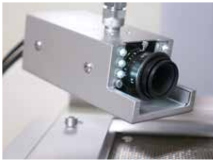
Reflow Process Camera (RPC) on the HR 550
