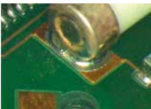
Lead-free assembly: non-wetting
