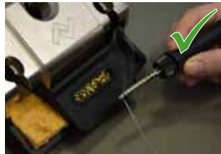
Add new solder after cleaning
