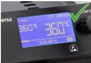
340 – 360 °C for lead-free solder
