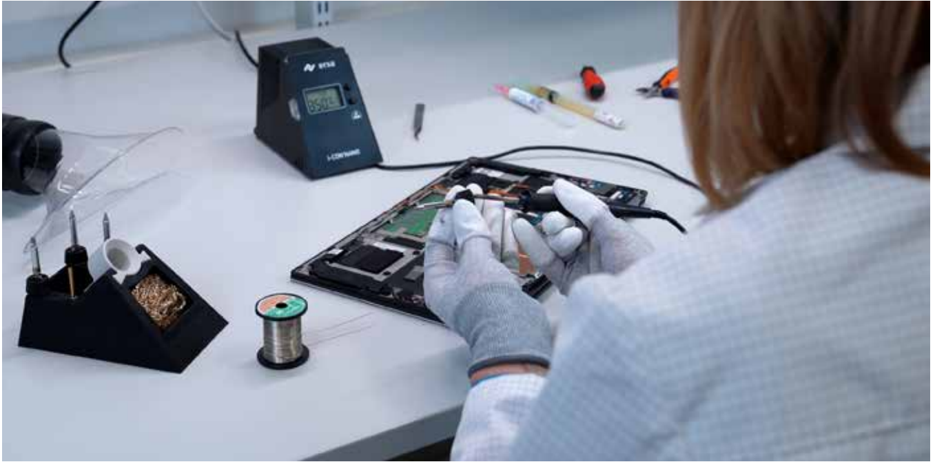
Changing the soldering tip of i-TOOL NANO MK2 is quick and easy.
