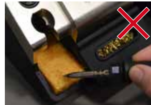
DAMP – NOT WET!
