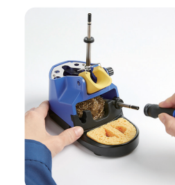
Removing a tip with the right groove of the attachment
