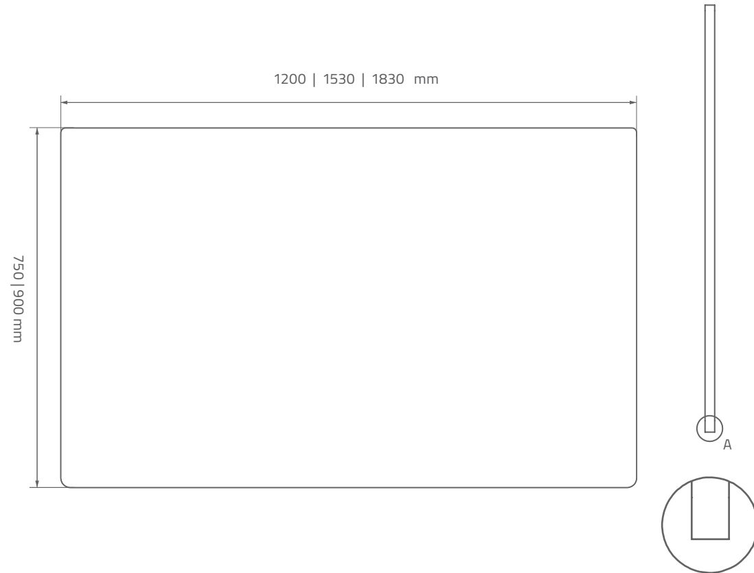
Rectangular HPL worktop with a depth of 750 mm
