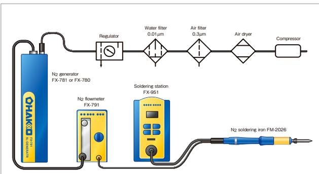
\* It is capable to supply high concentration nitrogen of 99.9% at the output rate approx. 1L/min. (at air supply pressure of 0.7MPa)
