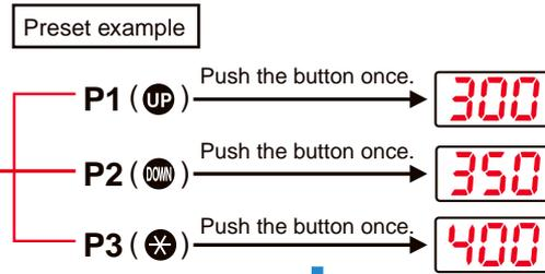
One push of a button can quickly recall each setting.
