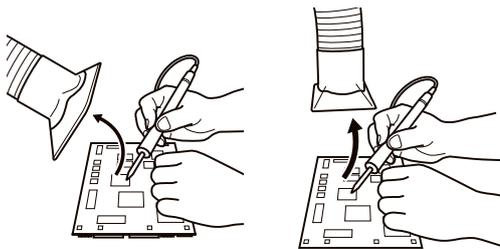
If the duct is mounted at an angle above the workpiece, it is affected by air conditioning.
