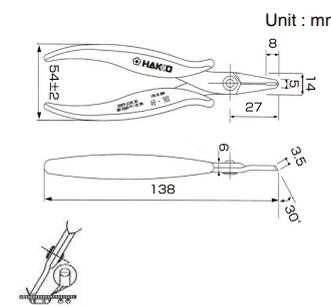
Cutting tool for flush cut
