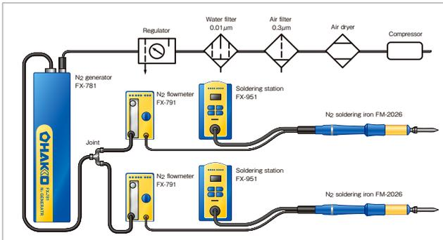
\* It is capable to supply high concentration nitrogen of 97% at the output rate approx. 1L/min. (at air supply pressure of 0.5MPa)
