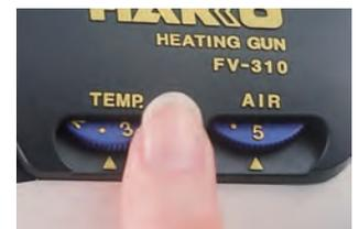
Although there is a click feeling, adjustment is stepless. Temperature and airflow suitable for the work can be set.
