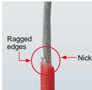
Conventional wire stripper could make ragged edges of insulation or damage strands.
