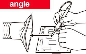
Duct is mounted on the worktable to provide excellent suction performance.
