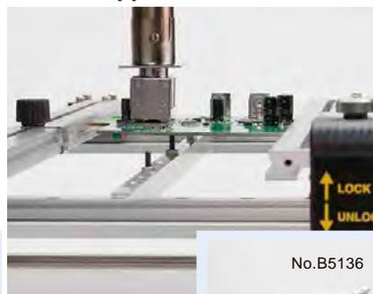
Supports P.W.B. from underneath to minimize its warping.
