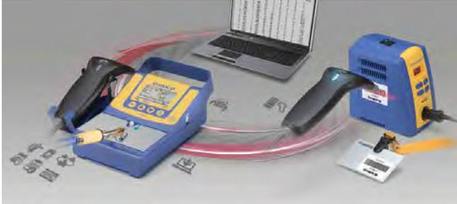
1. Scan the unit and the measurer's ID by a barcode reader.
