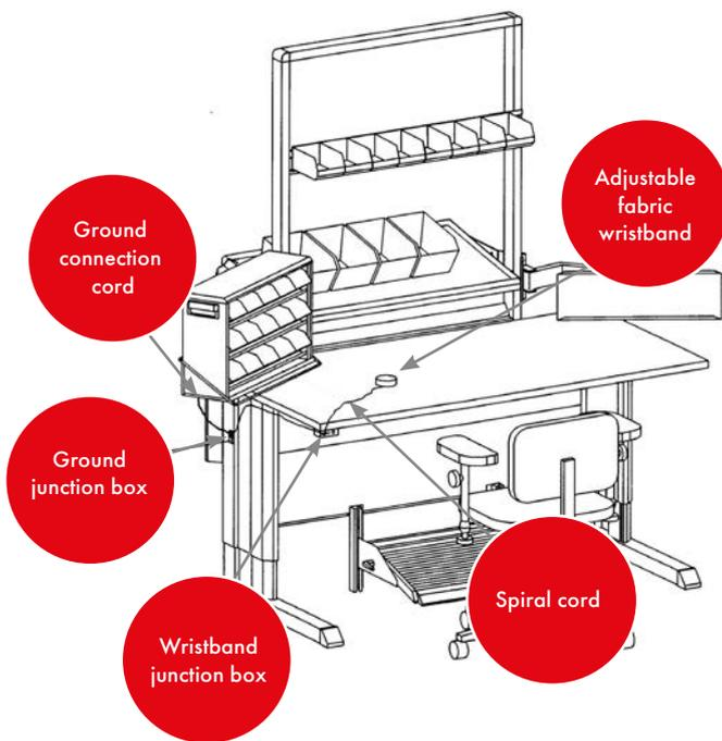
We have extensive experience in developing, manufacturing and supplying ESD furnishings. All our workstations and related products are available with an electrically semi-conductive coat of paint and we supply furnishings, seats and earthing components for ESD-protected workstations. We also build complete production systems equipped with ESD-protection. Our ESD-protected products meet the requirements specified in the IEC 61340-5-1 standard.
