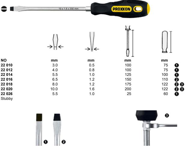
Matt-chrome plated blades of chrome vanadium special With hexagon flat for using an openend spanner as lever steel with precision black tip. (for sizes 8 and 10 on slotted and PH3 and PZ3 version).
