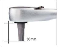
Fine tooth drive: Several of the 72 teeth engage simultaneously for transmitting high torque. 1/4" bit holder with magnetic insert. Distance between reverse lever and bit end only 30mm. Total length 120mm. Made from CrV steel, double nickel plated with matt chrome plated finish. Grip of oil and acid-resistant TPR (Thermoplastic Rubber). With practical hole for hanging up.
