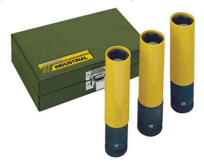
Sockets with plastic cover and plastic stop insert. For use with pneumatic screwdrivers 1/2". Made of high alloy special steel for superior wear resistance and a maximum torque of 500Nm. One piece each 17 - 19 and 21mm in sturdy steel box (powder coated).
