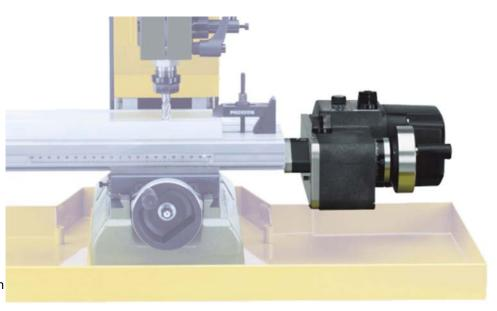
manual operation the handwheel needs to be mounted on the spindle of the drive-axis. Balanced special DC motor with electronic speed control (full-wave electronics). Manual drive with freewheeling function and two speed levels: Stage 1 for common machining (20 - 75mm/min). Stage 2: for machining at higher speed or quick adjustment of the X axis (90 – 260mm/min). Freewheeling function for manual operation by handwheel.
