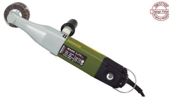
For grinding and finishing steel, non-ferrous metals and stainless steel surfaces.
