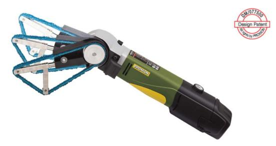
With continuously variable electronic speed control for constant speed even under high grinding pressure. The head can be angled by up to 60° at the push of a button. Suction connection with vacuum cleaner adapter permits clean working. Complete with four abrasive belts (2 x grit 80, 2 x grit 180) and two satin-finishing belts. Set includes lithium-ion battery Li/A2 (10.8V) and rapid battery charger LG/A.
