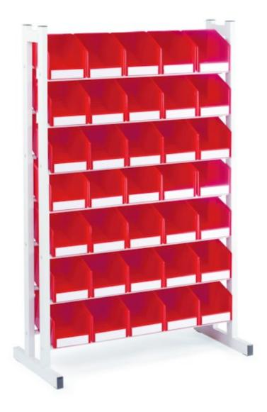
On BR stands, stacking bin are inclides at a 20-degree angle, enabling the excellent presentation of products. They offer an efficient storage system for daily use when small components are required frequently. This product includes a grey steel frame in an epoxy powder-coated finish and seven fixed, forward-slooping storage levels. Stacking bins must be ordered separately.
