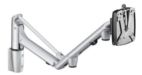
Highly ergonomic and easily height adjustable monitor arm with a gas spring. Easy mounting of the monitor with a quick- release mechanism, standard flat screen mount  $75 \times 75$  and  $100 \times 100$  for LCD screens.
